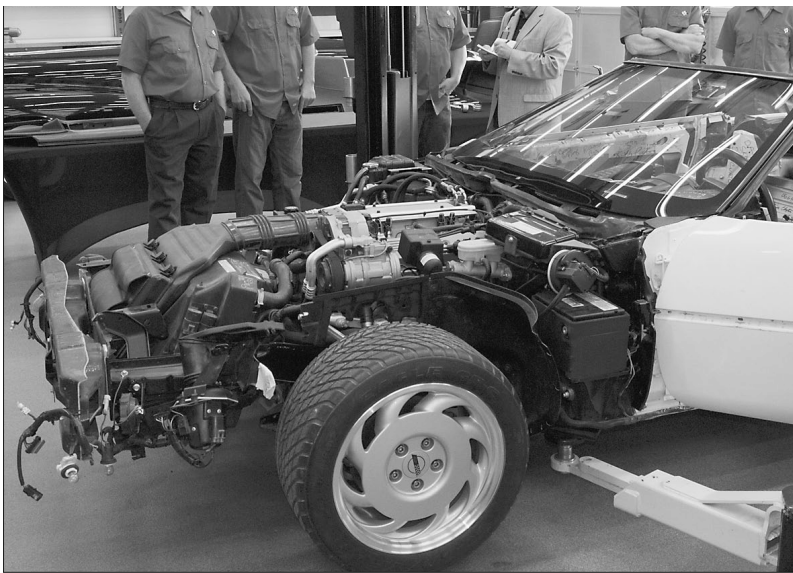
GM Design Center Technicians are repairing damaged, historic 'Vette.
